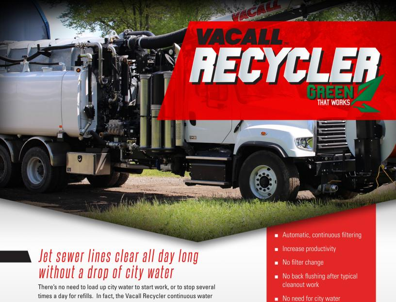
recycling system typically uses no city water at all for jetting.
